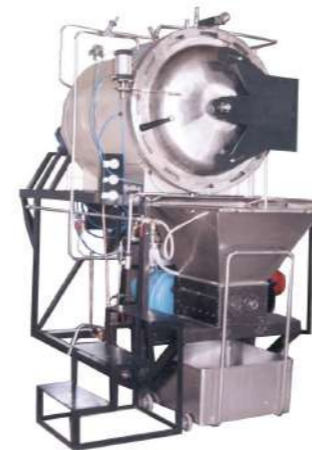
YSU-611 CYLINDRICAL MEDICAL WASTE STERILIZER WITH SHREDDER
